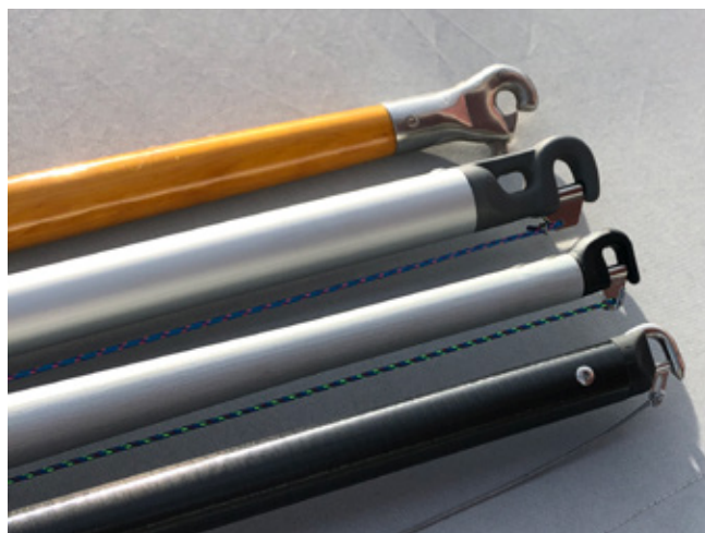
Spinnaker poles old and new- wood, aluminum and carbon fiber.
