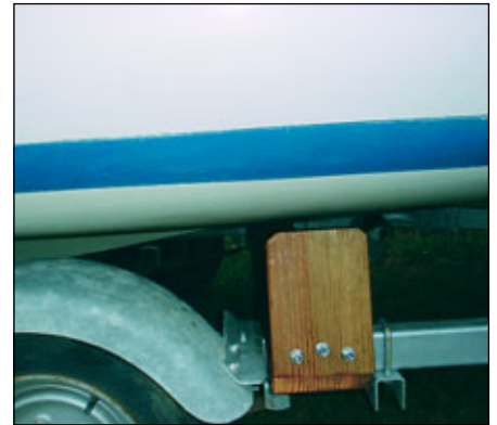
In designing the final step length, you must pay attention to the clearance to the hull.
