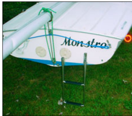
It is possible to mount the ladder even with access ports already on the transom.
