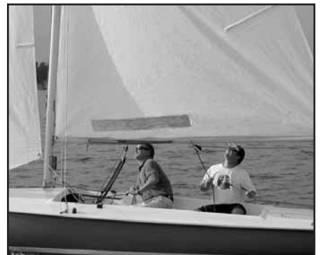
Cross-Cockpit Jib Sheeting and Hand-Held Mainsheet
