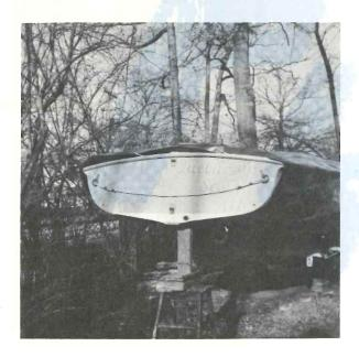
A REMINDER - To install a safety line between the two mooring rings, for use in case of capsize. (1/2" nylon shown)
